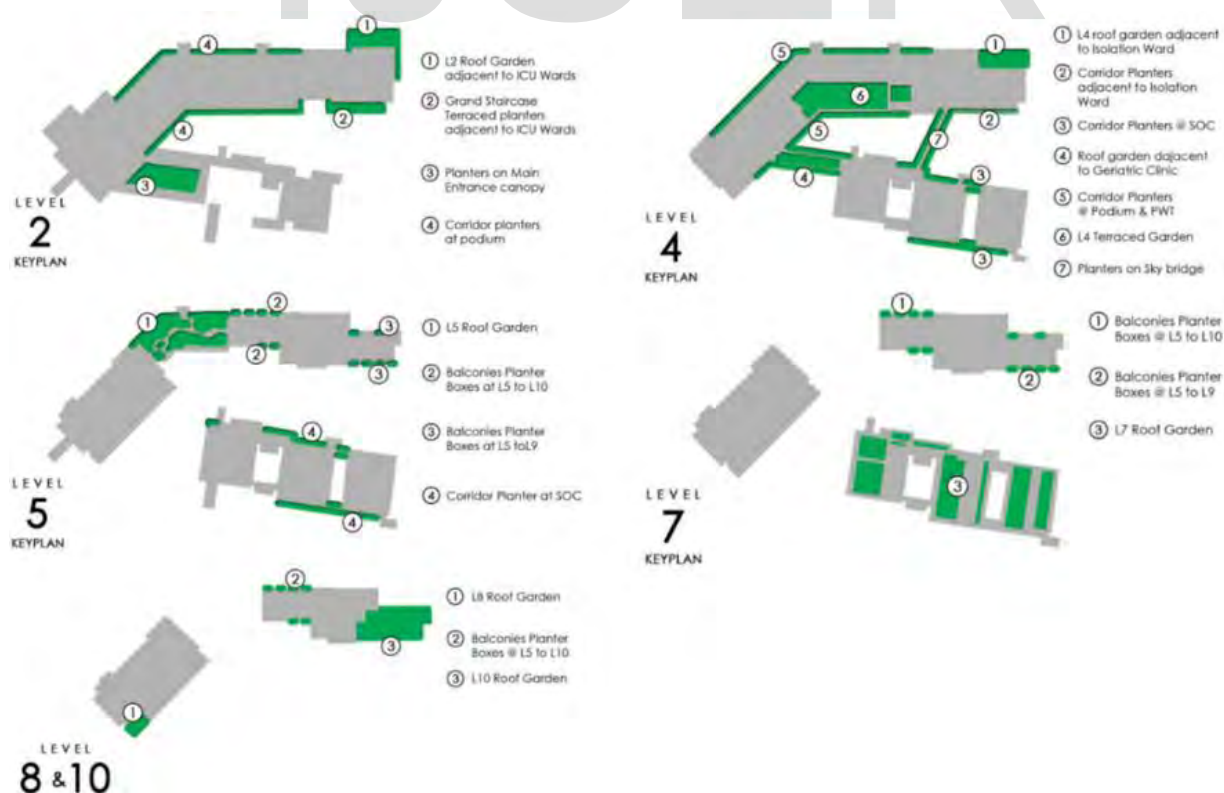
Fig. 4.4.4 Analytical key plans showing foot-print of greenery at every level of KTPH
