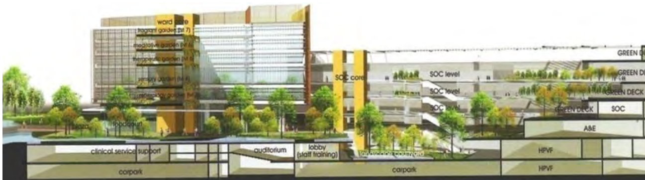
Fig. 1.3 Schematic section of Khoo Teck Puat Hospital, Yishun, Singapore demonstrates achieving day lighting, plants, natural ventilation and good air quality through courtyard design
